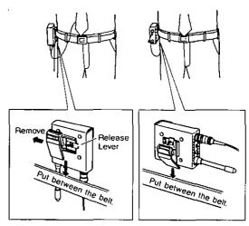
The Belt Case Clip can be mounted in a vertical or horizontal direction.
