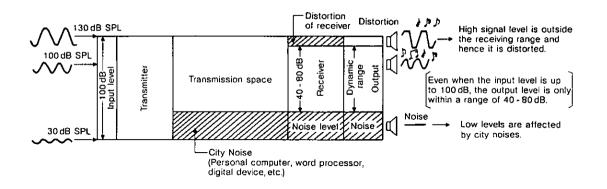
The Panasonic wireless system uses a compression / expansion technique to reduce the dynamic range of the audio signal before transmission. The signal is then expanded back to its original form at the receiver.
